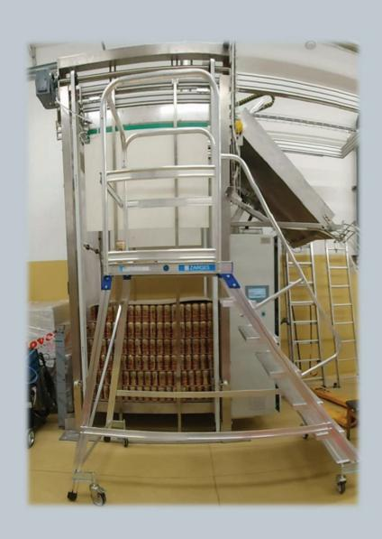
High-level bottle de-palletizer. Pallet with bottles is lifted to fixed high level conveyor and swept to it. Interlayer is automatically removed and stored in size magazine. Bottles continuous to conveyors.
