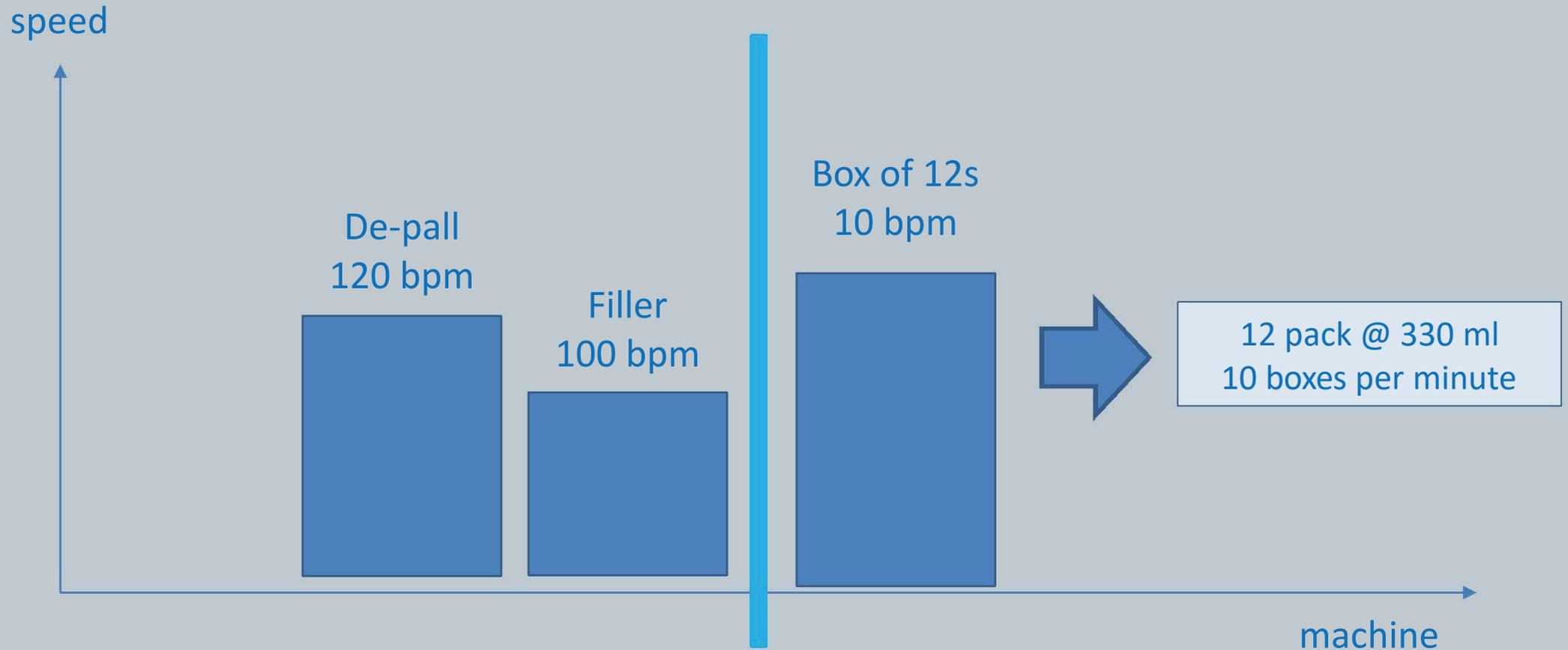
MACHINES CAPACITIES ARE CALCULATED BASED ON V-GRAPH WITH INCREASE OF 7-12% WHAT IS MINIMUM GOOD ENGINEERING PRACTICE
