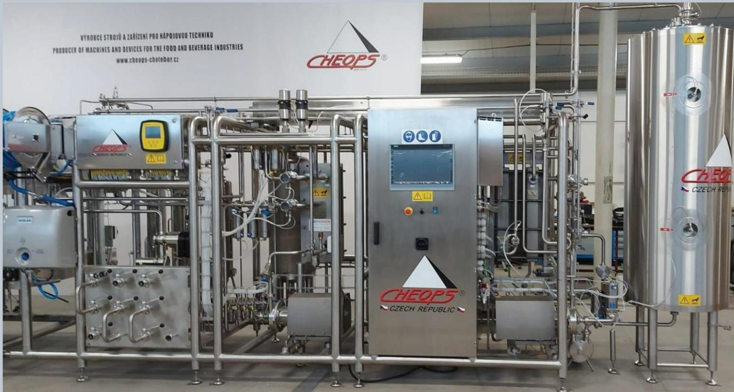
*Example of combined unit: CIP, flash pasteurizer, sterile filtration, carbonator, and nitrogenator*
