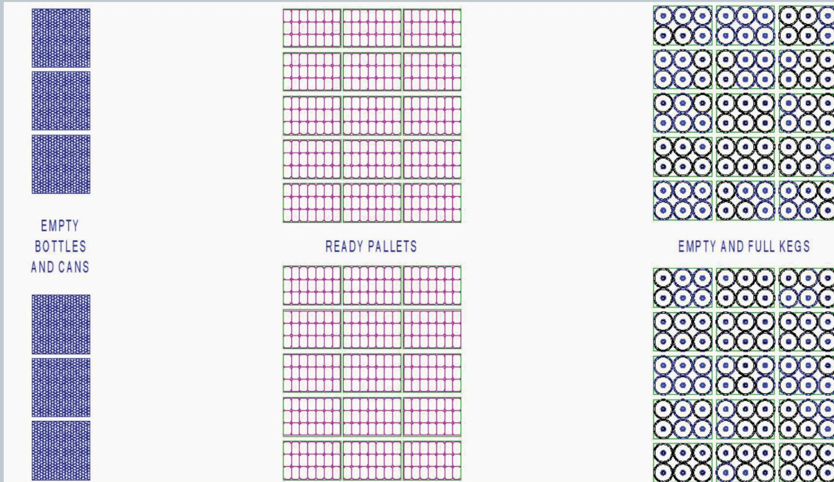
Sufficient warehousing area is needed. Not only for empty cans, ready pallets and kegs, but also for packaging material – clusters, trays, film for pallet wrapper etc. Total warehousing area needs to be calculated based on sales model and number of SKUs. This example is therefore illustrative.
